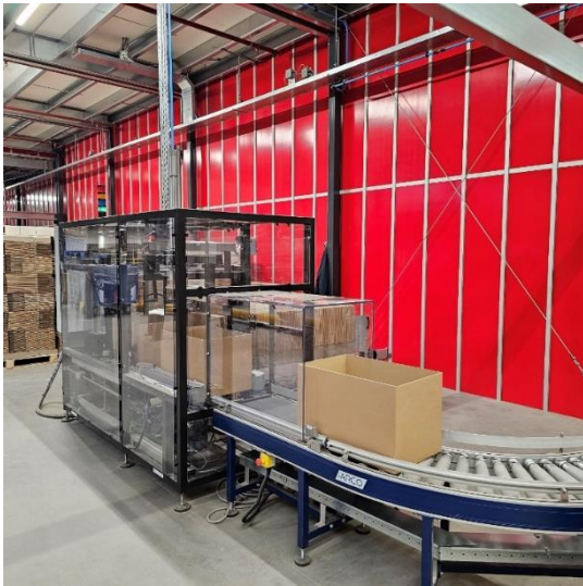
Cartons being formed by the automated Ranpak Form'it! box erector, ready for packing.
