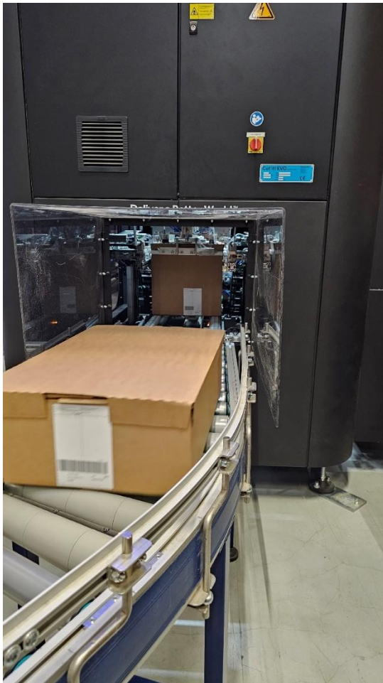
Securely sealed, right-sized carton exiting Ranpak Automation's Cut'it! EVO, ready for shipping.
